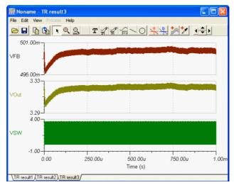
Why did the analysis run faster? Transient analysis was already preceded by the Steady State Analysis and the main capacitor's initial values (called Initial DC voltage in the Capacitor property box) was already set to the final DC voltage. For example, if you double-click on the C3 capacitor, you will see that the Initial DC voltage is already set to 3.31 V. Similarly, all the larger capacitor's initial values are set.
