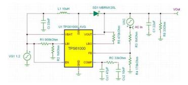
Note the VAC generator which is providing signal for the AC analysis., and the AC In Voltage pin which is the Input of the AC analysis (its IO state parameter is set to Input).
