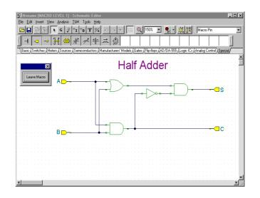
To do this, insert the newly created Half Adder twice into a new circuit and then add the additional components and wires as shown in the following picture.
