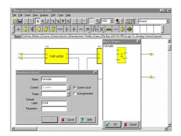
Note that in order to see the predefined symbols, the Macro Pin Label names must exactly match the names in the symbol. In our example, they must be (A, B, Ci, Co, S). If you do not see the symbol shown in the figure above, check the terminal names or try to recreate the symbol as shown later at "Making your own schematic symbols".
