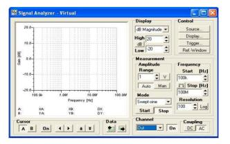
A useful feature of virtual instruments of TINA is that they take over the settings of the Analysis menu. Therefore, in our case, press the Start button of the Signal Analyzer and the amplitude Bode diagram will appear as shown in the figure below:
