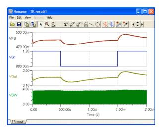
According to the waveforms, the input voltage will decrease from 1.2V to 0.8V for a T2=1ms time; and the starting edge (T1) and the ending edge (T3) of the pulse are 10us.
