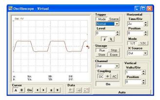
The wave is moving on the screen because by default the Oscilloscope is Auto (free running) mode. To synchronize the waveform select Normal mode with the list box below the Trigger field. The waveform will stop moving on the Oscilloscope. You can trigger the waveform
