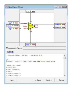
Take a moment to check the connections and if necessary correct them by dragging the connection labels.
