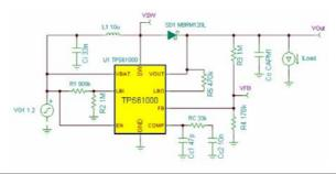
If you double-click on the ILoad generator and check its waveform, you will see that the DC part is 5mA while the pulse is 45mA in amplitude and 1ms in width.
