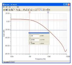
You can read exact input/output values by enabling one or more of the cursors, pressing the sea and/or sea and clicking on the curve where you want to run the cursor(s). If you run two cursors you can see the difference of the frequencies and values measured by the two cursors as shown in the figure below.
