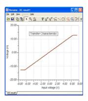
Type "Transfer Characteristic" and click the  $\boxed{}$  icon. Now you can position and drop the text into the diagram.
