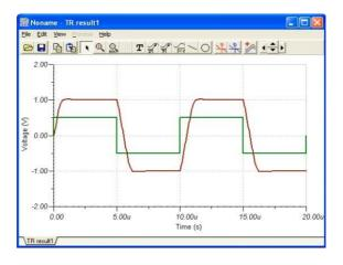
Change the End Display parameter to 20 u then press OK. In a separate window the transient response waveforms will appear. Exact input/output data points can be read by enabling the sea and/or separate graphic cursors.
