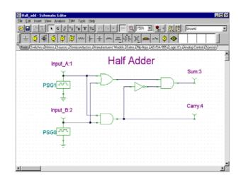
Delete the old terminals and replace them with subcircuit terminals, called Macro Pins in *TINA*. You can find and select the Macro Pins under the Special component toolbar.
