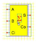
You should assign terminal names as shown in the picture below.
