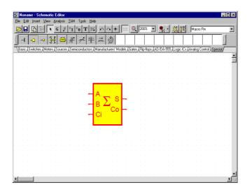
Double click on the symbol and the schematic inside the circuit will appear, showing two of our previous half adder macros. You can then double click on either of the macros to see the schematic inside. Return to the Full Adder and the main circuit by clicking the Leave Macro button.
