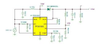
In this Boost Converter circuit the VG1 input line voltage is 1,2V. This is converted by the SMPS circuit to 3,3V.
