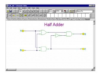
When you place Macro Pins, labels (such as Pin1, Pin2 etc.) are pre-filled in. Double click the Macro Pin and type in the new name in the label field. You can also drag the component with the mouse, or rotate it with the [+] and [-] keys or the pop+ buttons.
