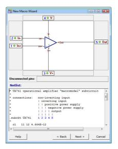
The dialog shows how the pin names on the graphic symbol are associated with the Spice node names in the macro. It also shows the text of the macro so you can check that the connections are properly made. If not, you can drag the macro node names to any terminal. However if all the pins are connected with a node number, then most likely the association is correct.
