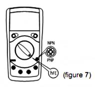
To measure transistor, set up the Meter as follows:
