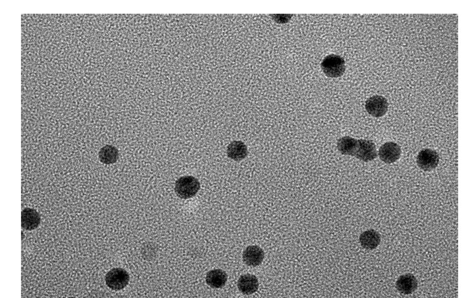
temperature had no negative effect on the size distribution of the nanoparticles, with the colloid forming almost instantly.
