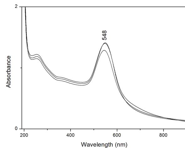
Fig. 1 UV-Vis spectra of the as synthesized nanoparticles
