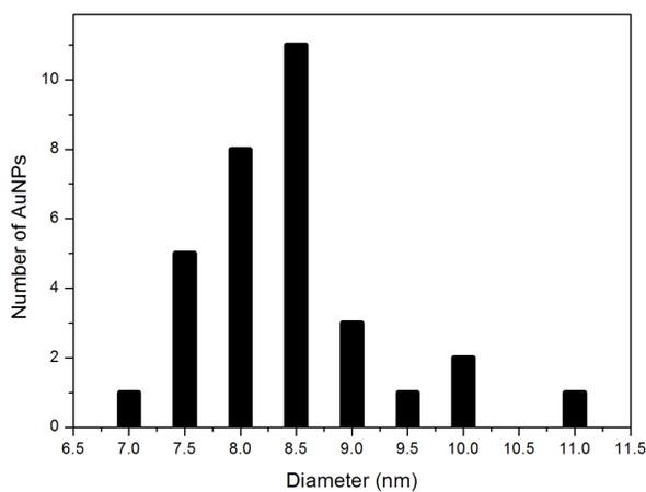
Fig. 3 Distribution of nanoparticle diameters gathered from TEM micrographs of the nanoparticles
