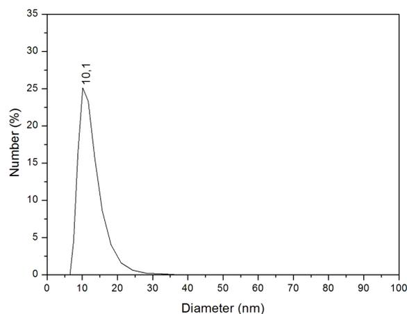
Fig. 4 DLS spectra of the as synthesized nanoparticles showing size distribution throughout the whole colloid
