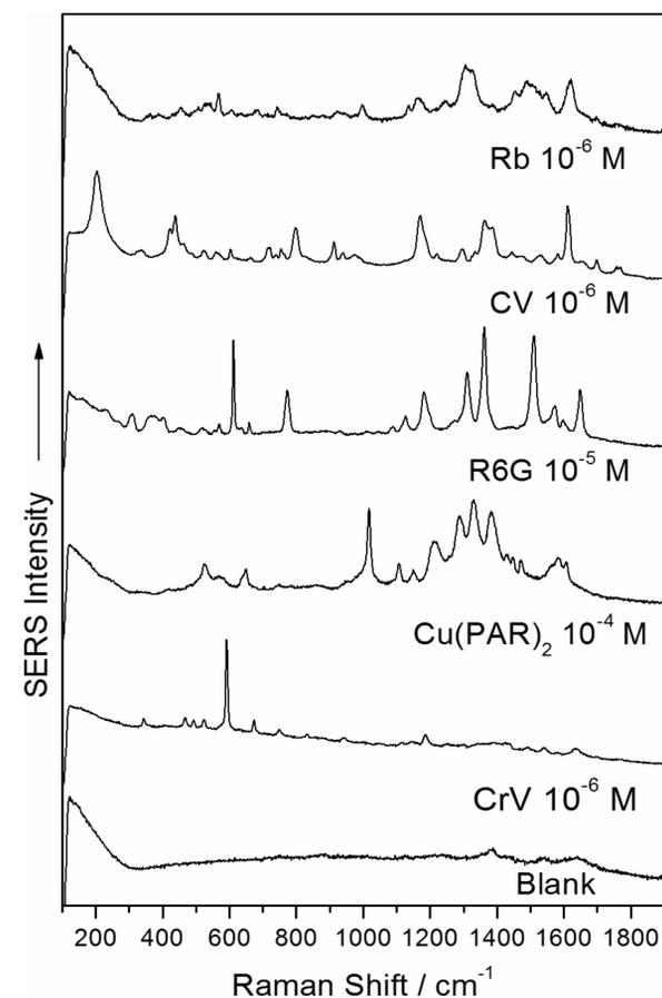
Fig. 5 SERS spectra of several analytes in micromolar concentrations with the as synthesized nanoparticles acting as a substrate
