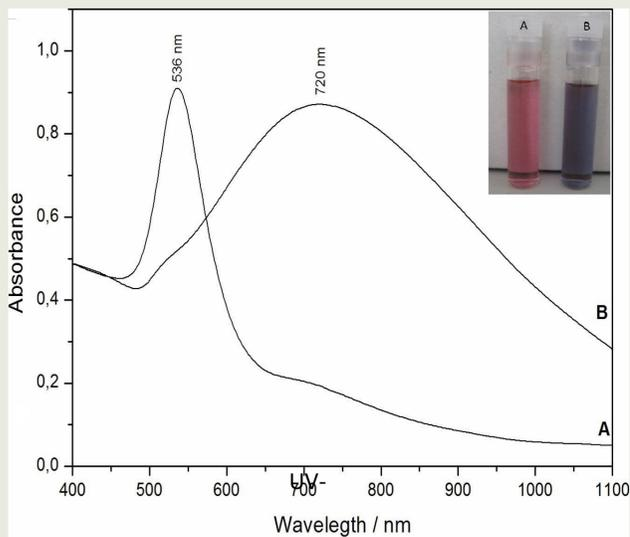
UV-Vis spectra of hydroxylamine reduced GNPs, accordingly to 20nm NPA and 120 nm NPA. The inset image shows a picture of the two colloids
