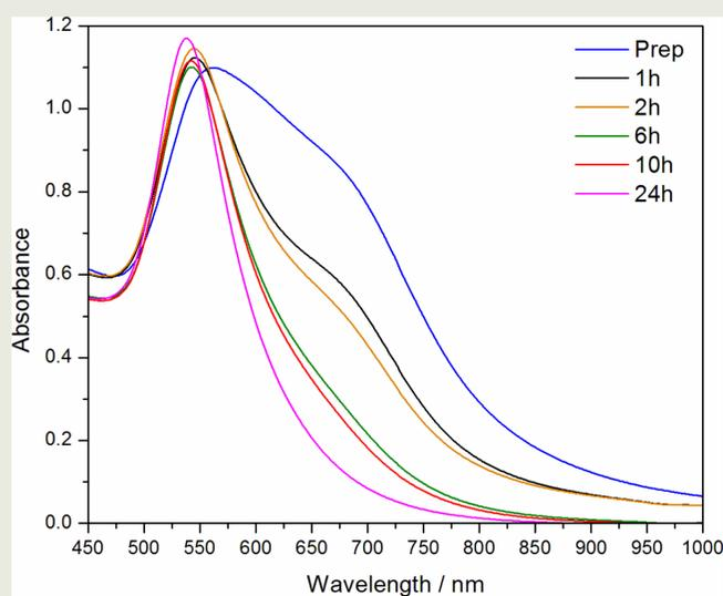
UV-Vis spectra of the 20 nm NPAs at different phases of the reduction process.
