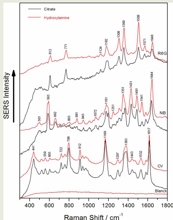
SERS spectra of Crystal Violet (CV), Niel Blue (NB) and Rhodamine 6G (R6G) obtained by using hydroxylamine (h) (CV  $10^{-7}$ M, NB  $5 \times 10^{-7}$ M, R6G  $10^{-7}$ M) and citrate (c) (CV  $10^{-6}$ M, NB  $10^{-6}$ M, R6G  $10^{-6}$ M) reduced gold colloids.
